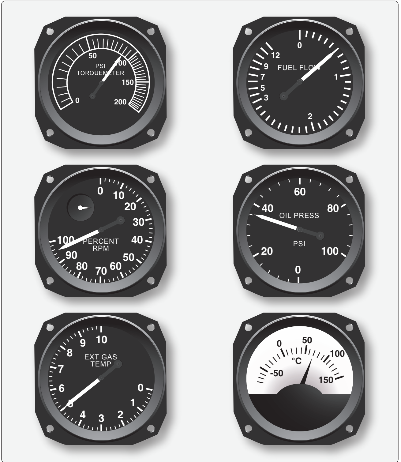
Figure 10-73. Typical turbine engine instruments.
