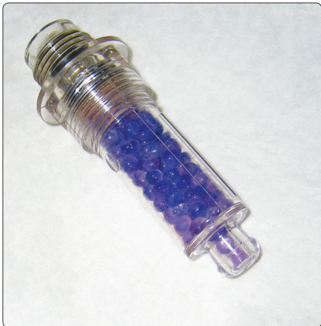
Figure 8-19. Dehydrator plug “blue” showing low humidity (Sacramento Sky Ranch).
