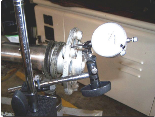
Figure 10-10. Checking crankshaft runout.
